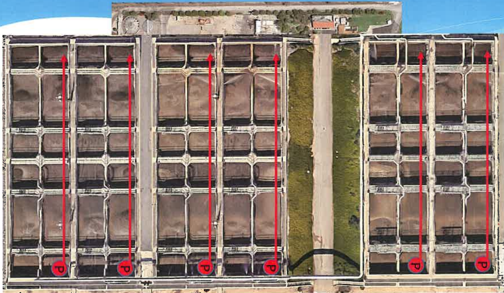
RP-1 Mixed Liquor Return Pump Locations
