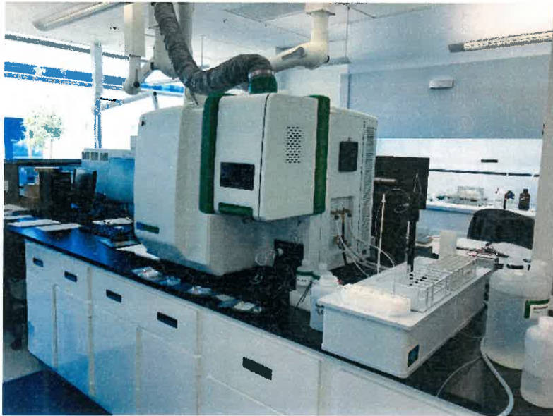
Inductively Coupled Plasma Spectrometer (Metals analyses)
