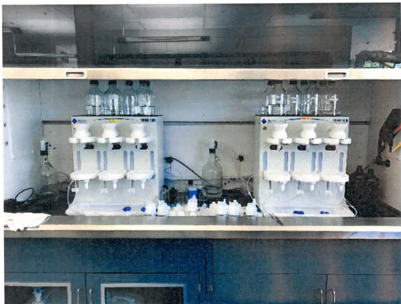
Solid Phase Extractors (Organics extractions)
