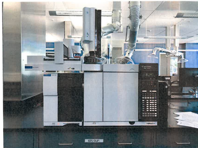
Gas Chromatograph/Mass Spectrometer (Semivolatiles and Volatiles)
