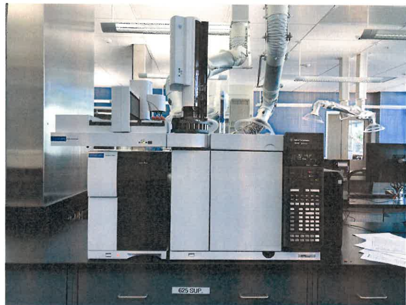
Gas Chromatograph/Mass Spectrometer (Semivolatiles and Volatiles)
