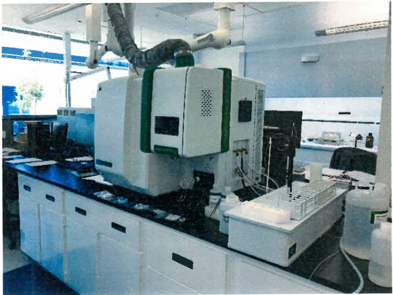
Inductively Coupled Plasma Spectrometer (Metals analyses)
