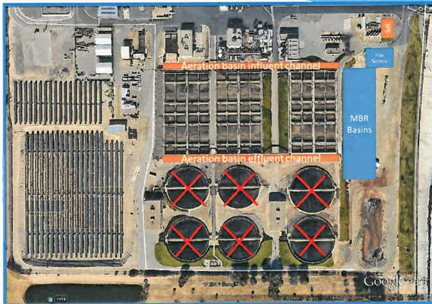
Alternative No. 4: MBR Retrofit without Additional Train
