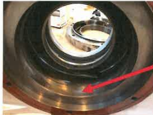
Bearing housing shows surface gouging caused by bearing that spun in place
