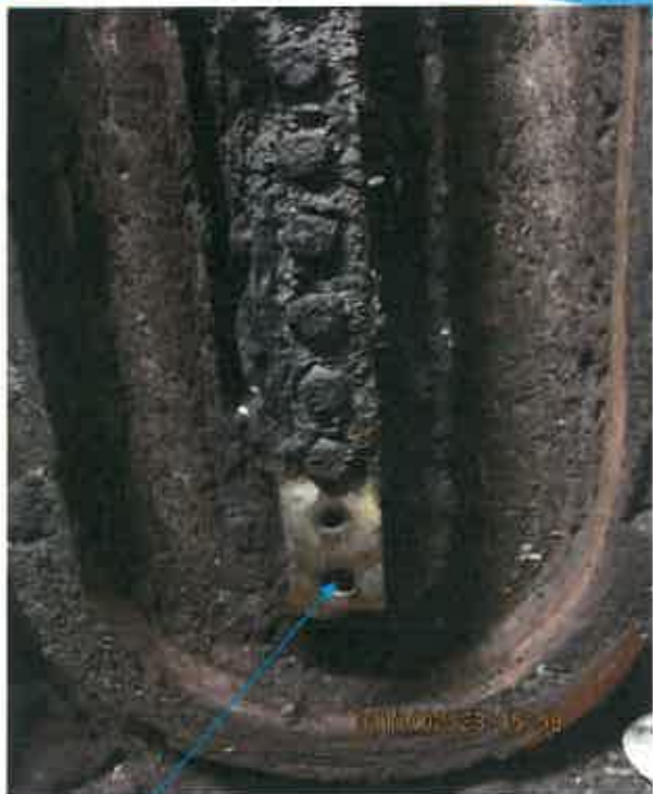
Track and Pin Rack Assembly wearing, allowing pins to fall out
