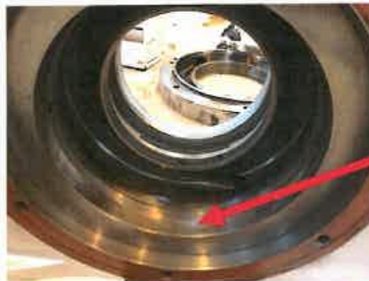
Bearing housing shows surface gouging caused by bearing that spun in place
