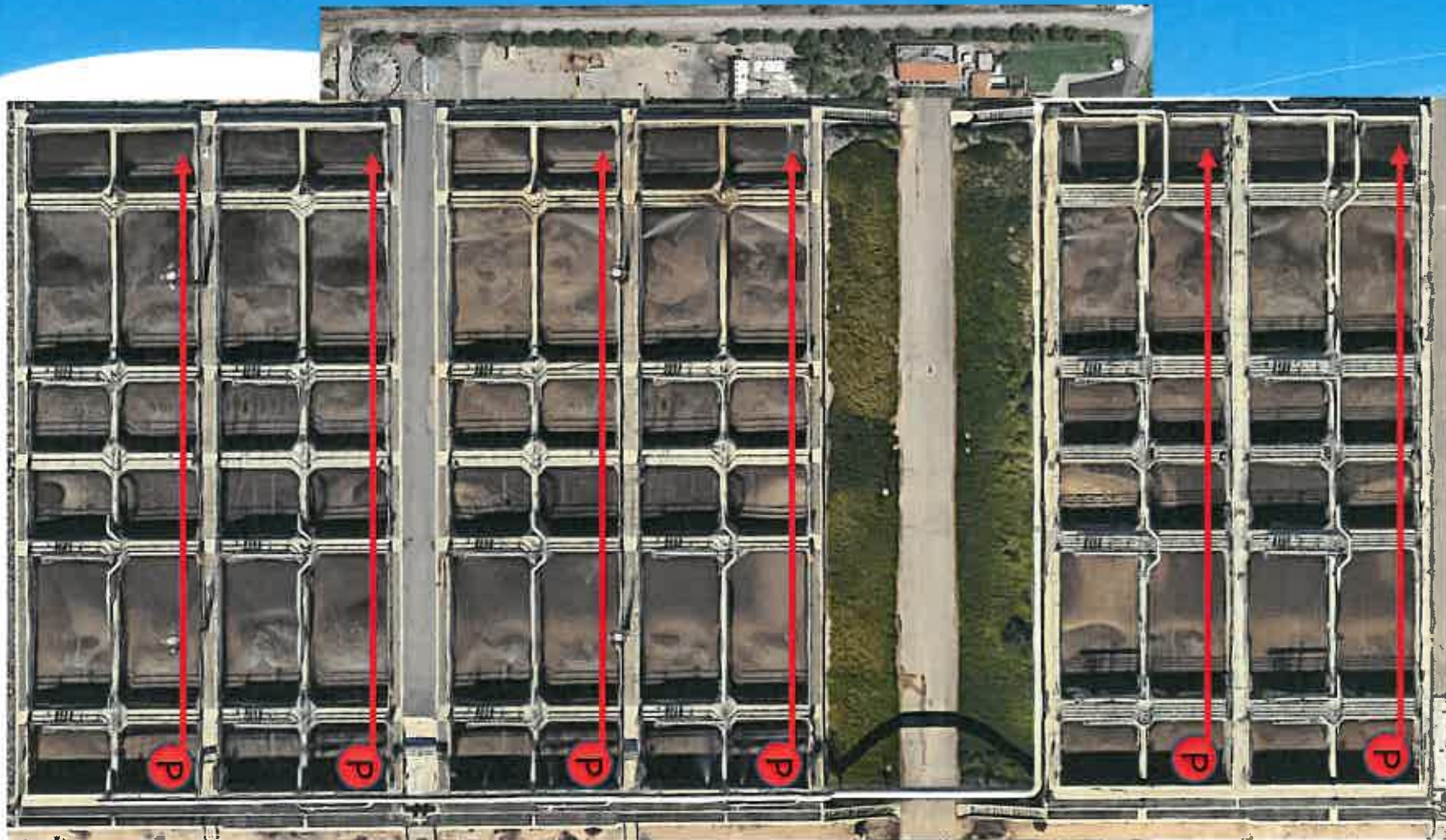
MLR Mixed Liquor Return Pump Locations
